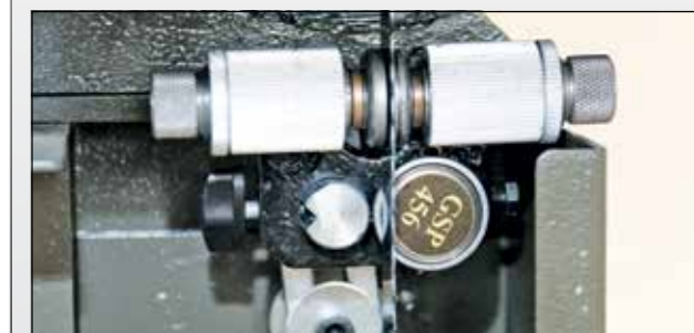
The lower guides are easily accessible
