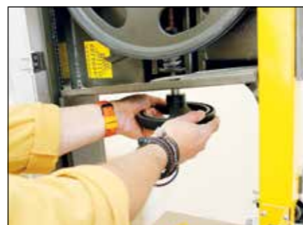
I found the tensioning wheel to be large and easy to operate
