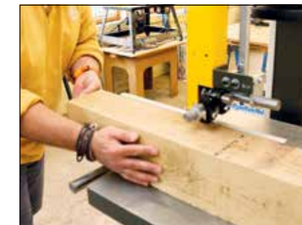
Cutting this wet oak caused the saw to slow as it clogged in the cut
