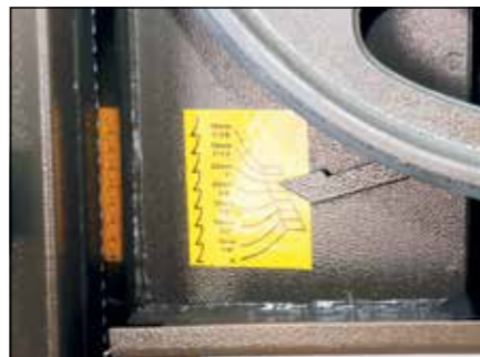
A basic needle indicates the tension setting. The top door has a viewing window to check this
