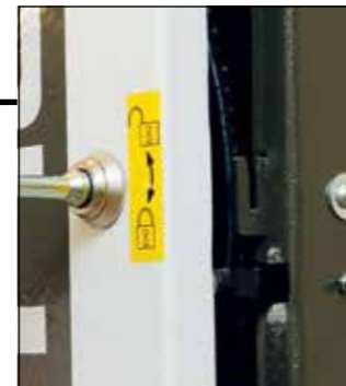
Each door is microswitched but still has a lock to secure it
