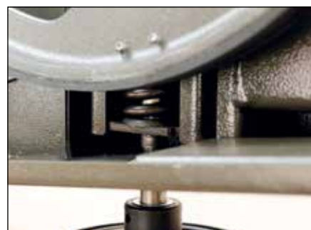
The heavy tension spring is just visible behind the cast band wheel
